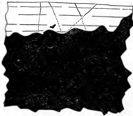
FIG. 7.—Galena block replacing limestone from Leadville, Colorado, showing wavy line of demarcation between galena (black) and limestone (white). About half natural size.
